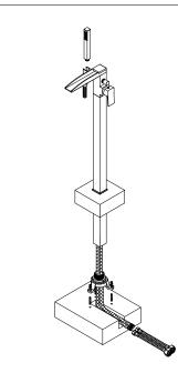
Please check that your pressure is suitable for this product before installation, details can be found on our website, recommed minimum working pressure: 0.5 bar, maximum working pressure: 3 bar
